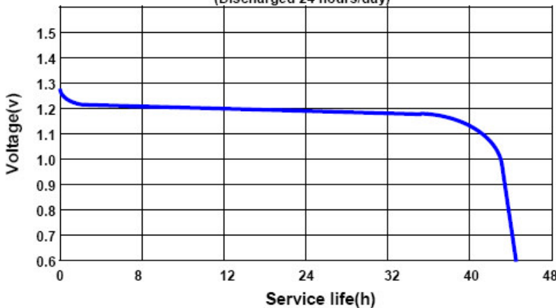
DISCHARGE CHARACTERISTICS AT 100Ω 25°C 60%RH (Discharged 24 hours/day)
