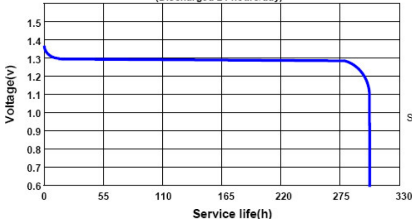
DISCHARGE CHARACTERISTICS AT 620Ω 25°C 60%RH (Discharged 24 hours/day)
